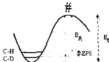
The maximum possible size of this effect is obtained if it is assumed that isotopic substitution has no effect on the energy of the transition state.
