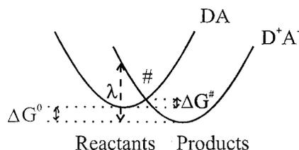
Here the reactants are shown as the donor/acceptor (DA) encounter complex, and the products the  $D^+A^-$  encounter complex.  $\Delta G^\ddagger$  and  $\Delta G^0$  are the free energy of activation and the standard free energy change in the reaction respectively.  $\lambda$  is the new quantity, the reorganisation energy.
