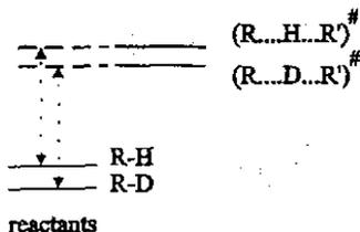
Now the difference in activation energies is less than the difference in the zero-point energies – the kinetic isotope effect is diminished in size.
